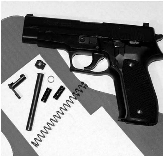
LaserMax® Combat Laser Sight, shown installed on this Sig P226 and disassembled at left. This unit utilizes a Class IIIa laser and produces a pulsing red dot. Power output is between 3-4mW.
